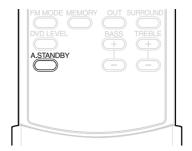
If there is no operation for 3 minutes while the disc is stopped, the power will be automatically turned off.
